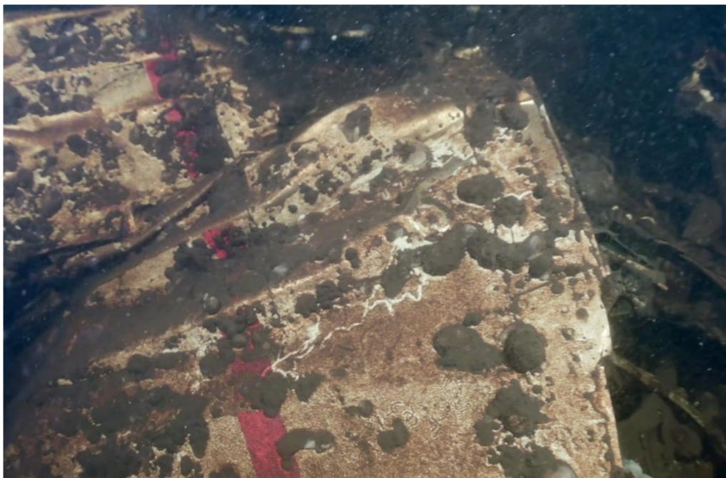
Figure 6: Vertical red propeller warning stripes on the port side of the forward fuselage. Frame from video: Maxwell Hohn
