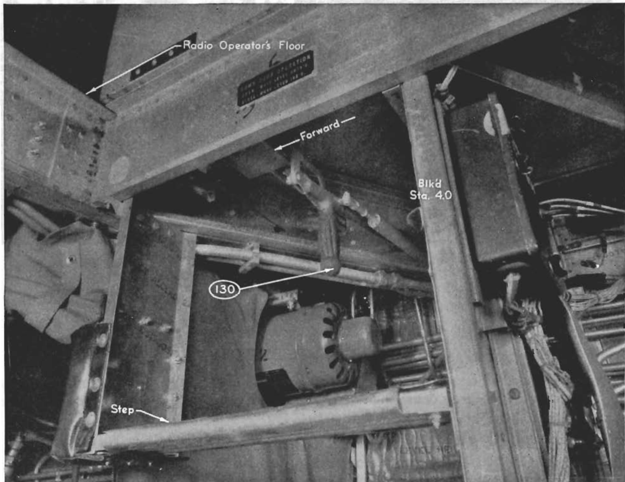
130. Auxiliary Bomb Door Handle (Inside View)
